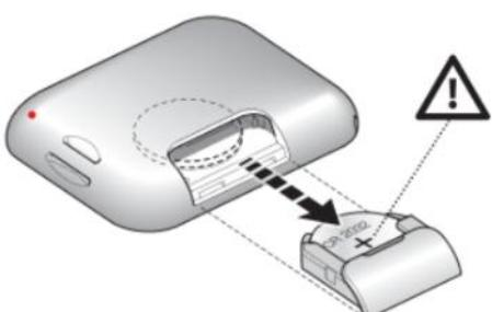
The battery is a CR2032 Lithium coin battery which must be inserted with the + symbol facing upwards as shown. These batteries are readily available online or from local outlets. If the fob still doesn't work after a new battery is fitted, it may need to be reprogrammed and you should contact the Managing Agent for this.
