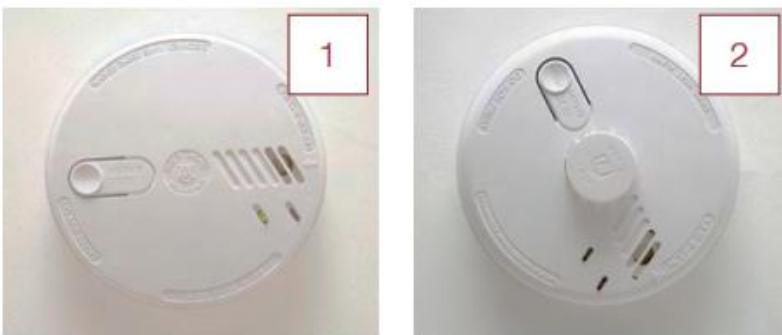
Smoke detectors (Picture 1) are installed in various locations including bedrooms and hallways, with a Heat Detector (Picture 2) in the kitchen. Both types are mains operated with a back-up battery. Each unit should be tested regularly by pressing the TEST button and batteries replaced when necessary. If the detector beeps once every 60 seconds, the battery needs replacing.
