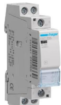
The contactors are Hager ESC225 and are available from most electrical suppliers for about £25-30 each. **Ask a qualified electrician to fit them** - and make sure they fit Heat Dissipation Inserts (spacers) between them, and between the contactor and the hot water time switch.
