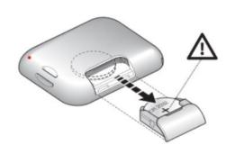
The battery is a CR2032 Lithium coin battery which must be insterted with the + symbol facing upwards as shown. These batteries are readily available online or from local outlets If the fob still doesn't work after a new battery is fitted, it may need to be reprogrammed and you should contact the Managing Agent for this.
