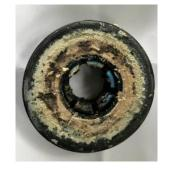
If water is seen to be running continuously into the toilet, the most likely cause is a build-up of limescale on the valve seal in the cistern, preventing a watertight seal. It may be possible
